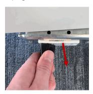
2. Using an antibacterial disinfecting wipe, gently wipe the controllers down. **DO NOT USE A DRIPPING WET CLOTH** – this may damage the internal electronics. Ensure you wipe each joystick, button, and switch on the boom and scissor controllers.
